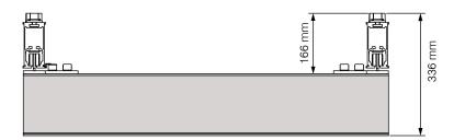
I. Rail C parallel rails with underhanging rail C traverse rail
